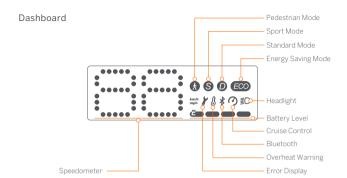
Speedometer: Display the current speed of the KickScooter, as well as error codes.
